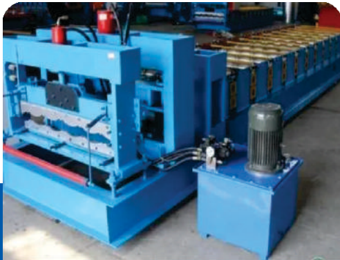
Roofing Sheets Roll Forming
